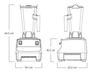
Includes Drink Machine Two-Speed with 1.4-liter high-impact, clear/stackable standard container, complete with Wet blade assembly and lid, and black base.
