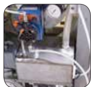
Oil tank with external fill and low level indicator
