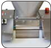
The drum can also be lubricated at each cycle after discharging the dough piece (Option)
