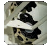
Bronze pinion ring no force exerted on the chain
