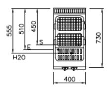
E = Electric H2O = Cold water Ø 3/4" S = Drain Ø 1"
